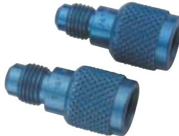
Liquid charging is recommended when charging blends into refrigeration and air conditioning systems. Since compressors cannot compress liquids, however, you need a liquid charger adapter for safe and fast liquid charging through the low pressure side of a system. The YELLOW JACKET adapter connects to the cylinder valve or refrigerant can.
