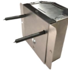
Use the external adapter plate when installing the Orion system to metal duct work. First rotate the probes 90 degrees. Use the supplied self tapping 10-32-1/4" screw. Attaching the plate ensures that there will be no air leakage from the duct work after the installation.
