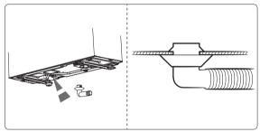
**4** Be sure to plug the rest of drain holes not connected with drain plugs using drain caps.
