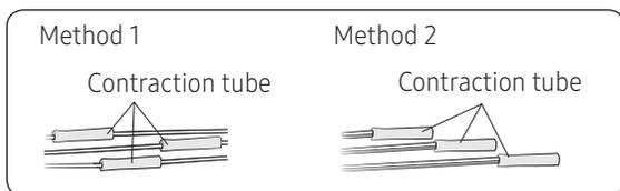
6 Wrap it with the insulation tape twice or more and position your contraction tube in the middle of the insulation tape.
