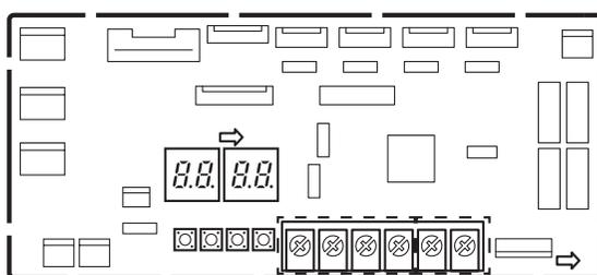
Do not connect the power and communication wires to these terminal blocks
