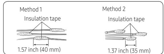
7 After tube contraction work is completed, wrap it with the insulation tape to finish.
