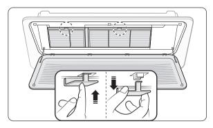
Press the Push signs  $(\nabla)$  on the air filter. Grab the handle of the air filter and pull it out from the indoor unit with your hand.
