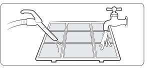
Clean the air filter with a vacuum cleaner or soft brush. If dust is too heavy, then rinse it with running water and dry it in a ventilated area.
