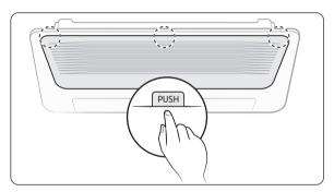
Press the **Push** signs on the front panel, then open the grille.
