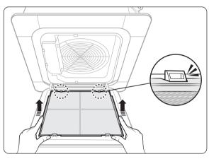
Pull out the air filter from the indoor unit.
