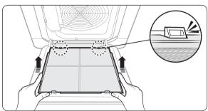
Pull out the air filter from the indoor unit.
