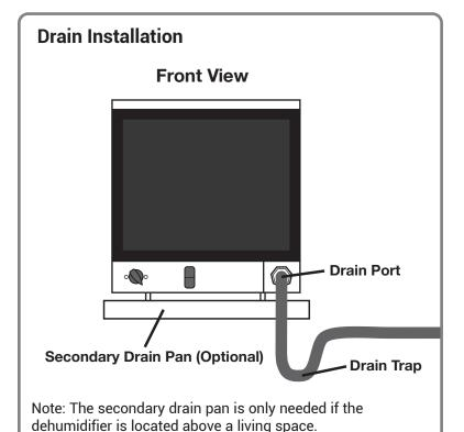
Use care to keep the hose as flat to the floor as possible after your trap is in place. Be sure the hose is not kinked or otherwise restricted so water can pass through the hose freely. Improper installation of the drain hose may result in water leakage.
