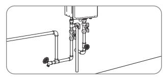
It is recommended to use unions and flexible copper connections at the COLD and HOT water lines. They allow the water heater to be disconnected easily for servicing.
