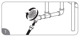
Disconnect drain hose. Make sure the drain valve is closed.
