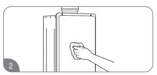
Clean the water heater and the remote control with a damp soft cloth and mild detergent. Gently wipe and completely dry all surfaces.
