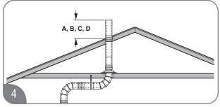
Determine the vent terminal height and install the vent pipe accordingly. Refer to "Vertical Vent Terminal Location" on this Use and Care Manual for clearance requirements.
