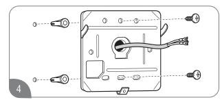
Install the base plate to the wall using suitable screws and wall anchors.
