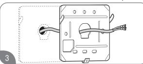
Feed the remote control cable through the large center hole in the base plate.
