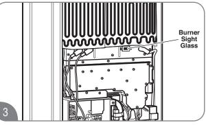
While the water heater is operating, inspect the main burner flames through the burner sight glass. The flames should be blue when the main burner is firing.
