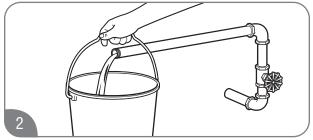
Before attaching the water line to the water heater, open the shut-off valve. Run the water until it has purged all contaminants (sand, debris, air, caulking).
