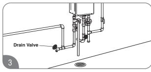
Drain the water heater. See "Draining the Water Heater" Section.
