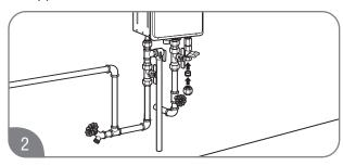
Install a ground joint union or ANSI design-certified semi-rigid or flexible gas appliance connector to the open end of the manual gas appliance shut-off valve. The (NFGC) ANSI Z223.1 and CAN/CSA B149.1 codes mandate the use of manual gas shut-off valves.
