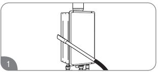
Vacuum around the water heater to remove any dust, dirt, and/or lint buildup.
