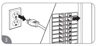
At least 10 seconds after Step 1, unplug the water heater or disconnect the power supply at the circuit breaker box.
