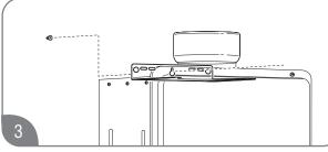
Position the upper mounting bracket and partially install the center mounting screw. The clearance between the screw head and the wall should be about 1/8 in. (0.3 cm). Hang the upper bracket on the screw.
