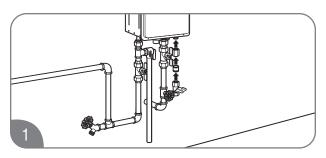
Install the manual gas appliance shut-off valve to the gas connection at the water heater. The shut-off is supplied with the water heater.
