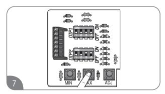
Push and hold "Max" button until "ON" is shown on the display of the remote control.
