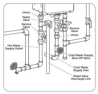
One end of the relief valve discharge line connects to the HOT water outlet pipe as shown above. The other end of the pipe should be routed to a suitable drain to eliminate potential water damage. For safe operation of the water heater, be sure that:
