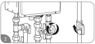
Close the gas shut-off valve(s).
