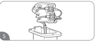
Secure the remote control extension cable on the hook located on the side of the remote control connection base.
