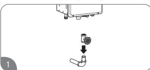
Install a COLD water shut-off valve near the inlet line on the water heater. This valve will be used for servicing and draining purposes.
