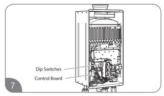
Find DIP Switch 2 in the top-right portion of the control board. The switch labeled "DIP 2" is the bottom switch.
