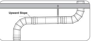
When a water heater is vented vertically, an UPWARD slope must always be used. Always attach a drain hose to the condensate collector and plumb the hose to a sanitary sewer drain.
