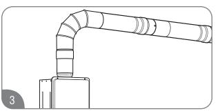
Attach required vent sections between the water heater collar and the horizontal vent termination.
