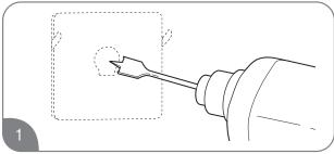
Drill a 1- to 1 1/2-in. (2.5/3.8-cm) hole at the proposed control location. Install the remote control cable between the location of the remote control and the water heater.
