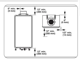
Minimum water heater clearances from combustible and noncombustible construction are as follows: - 1/2 in. (1.3 cm) for sides
