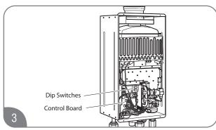
Find DIP Switch 1 located in the top-right portion at the control board. The switch labeled "DIP 1" is the top switch.
