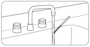
Turn on the hot water faucet and place a thermometer in the water stream.
