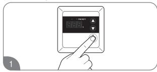
Turn off the water heater by pressing the POWER ON/OFF button on the control panel.
