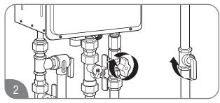
Close the gas shut-off valve(s).
