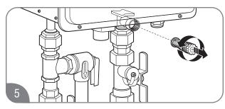
Close the shut-off valve and remove, clean, and replace the water filter.
