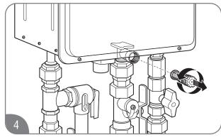
Unscrew the water filter from the base of the cold water inlet line and carefully slide it out of the line.
