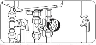
The water heater and its manual gas shut-off valve must be disconnected from the gas supply piping system whenever the pressure testing will exceed 1/2 psi (14 in. w.c. [3.5 kPa]).
