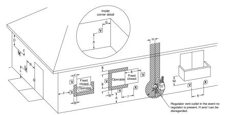
$\underline{W}$  vent terminal  $\otimes$  air supply inlet  $\underline{W}$  area where terminal is not permitted Horizontal Vent Terminal Location for Direct Vent
