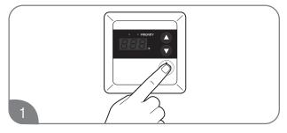
Turn off the water heater by pressing the POWER ON/OFF button on the control panel.
