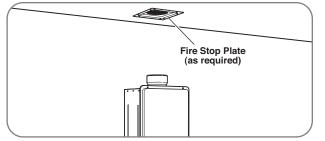
Every vent pipe penetration of a floor or ceiling that is not in a fire-rated shaft requires a fire stop plate.
