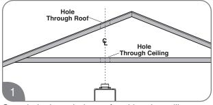
Cut a hole through the roof and interior ceiling to accommodate the vent pipe.
