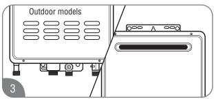
Check the air intake and vent outlet for blockage and/or debris.
