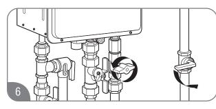
Open the gas shut-off valve(s).
