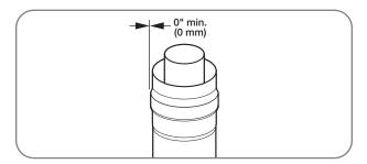
Minimum clearance around the coaxial vent pipe should meet the specifications listed on the instruction/warning label on the water heater. If no label is found, use the vent manufacturer's specifications or a minimum clearance of 0 in. (0 cm) around the vent pipe. General
