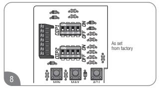
The factory setting for this switch should all be in the OFF position (DOWN).
