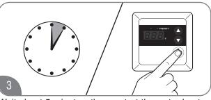
Wait about 5 minutes; then restart the water heater by pressing the POWER ON/OFF button.
