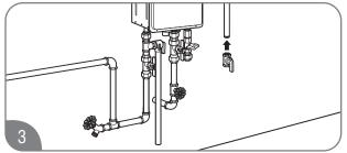
Install a manual gas supply line shut-off valve to the end of the gas supply line.
