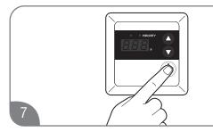
Press the POWER ON/OFF button on the control panel to restart the unit.
