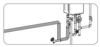
Long hot water lines should be insulated to conserve water and energy.
