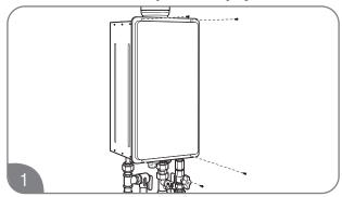
Remove 4 screws and the unit cover panel.
