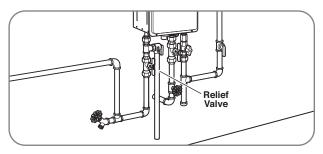
Annually check the operation of the pressure-relief valve. Lifting the lever handle on the pressure-relief valve opens the valve to flush hot water through the discharge line to the drain. After several gallons have drained, release the lever handle to close the valve and stop draining.
