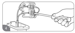
Firmly tighten the terminal screws by hand.
