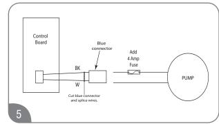
To connect to the pump, cut the blue connector, splice the wires, and add a 4 amp fuse to the hot wire of the pump.
