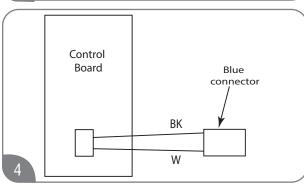
The wire harness for the recirculation pump is bundled with the wire harness from the control board. Find a blue connector with a black and a white wire.
