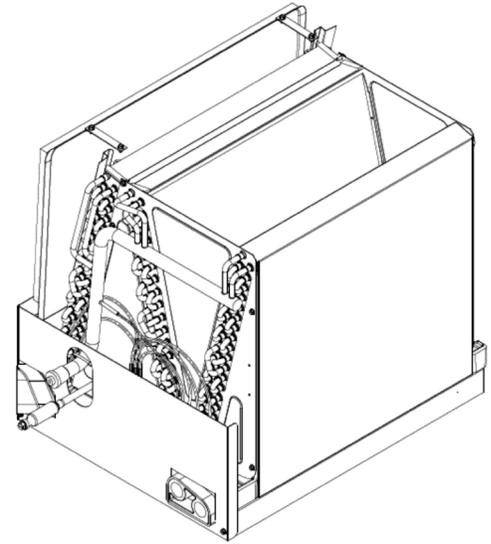
**NOTE:** Sliding the coil into the coil rail before attaching coil rack front.
