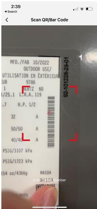
Figure 9. Scan the unit serial number barcode and verify it matches the ODU serial number at the rating plate of the unit to be reprogrammed. Then, click Continue.
