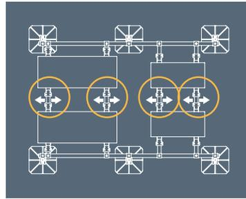
**Linear Adjustment** The cross bars supporting the equipment unit can slide along the end bars into position required, then be locked in place.
