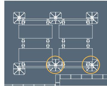
**Leg Assembly Positioning** The leg assembly is typically positioned outside the frame work, but can be placed inside the framework to avoid an obstruction.
