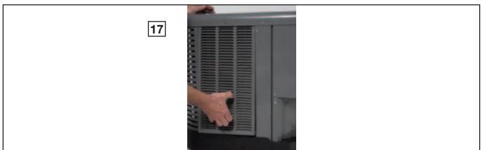
The outdoor fan motor has sleeve bearings and is inherently protected. The motor is totally enclosed for maximum protection from weather, dust and corrosion. Access to the outdoor fan is made by removing four fasteners from the fan grille. The outdoor fan can be removed from the fan grille by removing 4 fasteners in the rare case outdoor fan motor fails.
