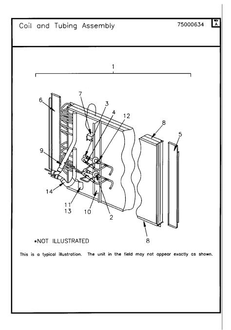
COIL & TUBING ASSEMBLY Parts List Number :TWEUP13B Model Number :TWE120B300BA
