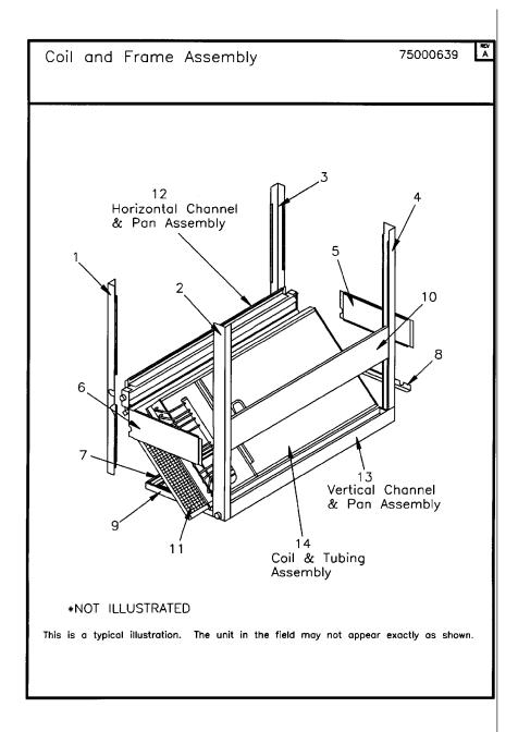
COIL FRAME ASSEMBLY Parts List Number :TWEUP13B Model Number :TWE120B300BA
