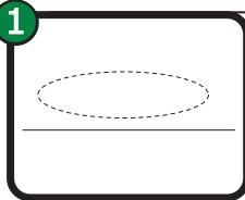
Cut a 3 1/8" hole through the outside soffit panel or use existing hole.
