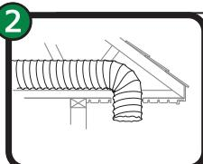
Starting from the exhaust source, feed the duct through the pre-cut soffit panel opening.
