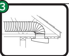
Attach duct to collar using a clamp (Not Included) and tighten. Insert the vent into pre-cut opening making sure the facing is flush against the soffit panel. Secure vent with screws (Not Included) to soffit and tighten to secure the vent.
