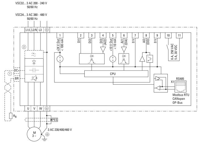
Figure 66. Block diagram VSC1D...NxA66...
