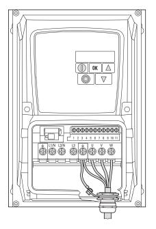
Figure 49. Grounding the EMC cable gland
