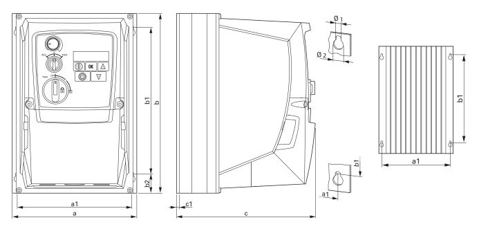
Figure 78. Dimensions for VSC with IP66 degree of protection (NEMA 4X)
