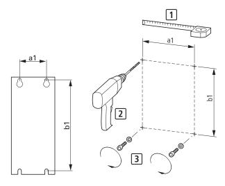
Figure 27. Mounting dimensions
