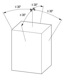
Figure 23. Mounting position
