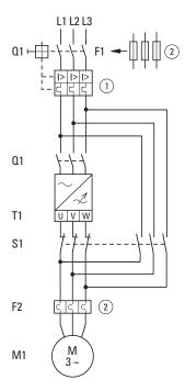
Figure 18. Bypass motor control (example)
