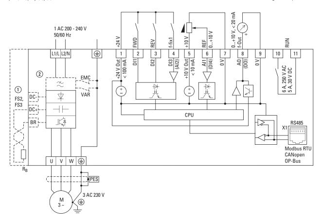
Figure 62. Block diagram VSC12...
