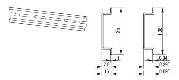
Figure 28. Mounting rail conforming with IEC/EN 60715
