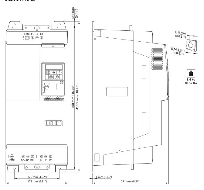
Figure 77. Dimensions and weight for VSC with frame size of FS4 and IP20 (NEMA 0) degree of protection
