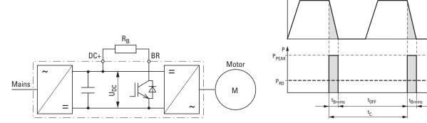
Figure 16. Braking cycle, fast motor stop with external brake resistor
