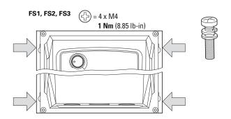
Figure 32. Openings for fixing screws
