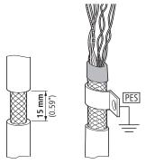
Figure 53. Screen termination at one end (PES) close to the variable speed drive
