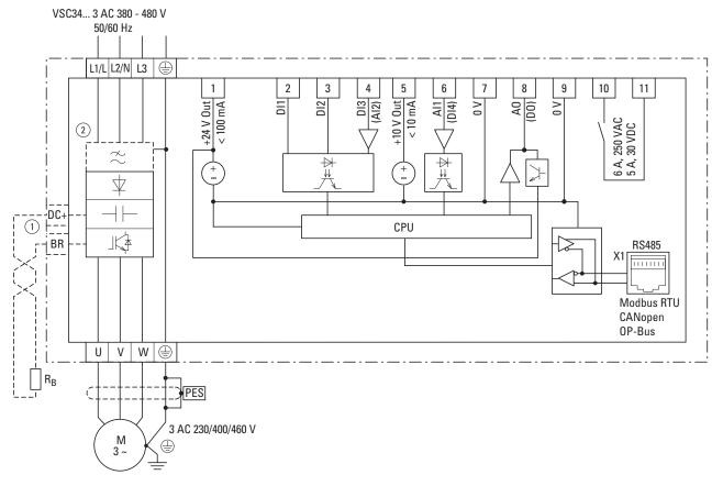
Figure 70. Block diagram VSC32...A66..., VSC34...A66...
