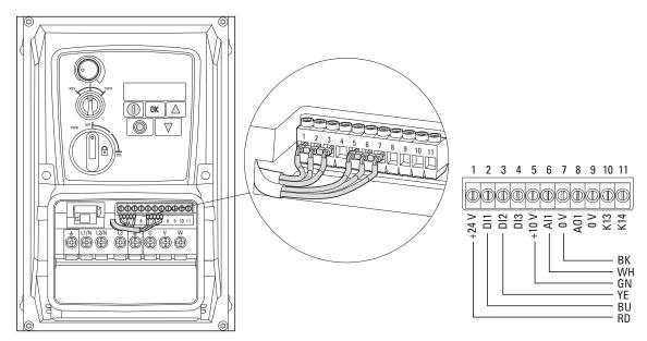
Figure 59. VSC...A6S... (connection wired at the factory)
