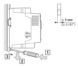
Figure 30. Dismantling from mounting rails
