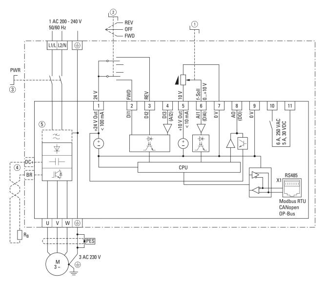
Figure 67. Block diagram VSC12...A6S...
