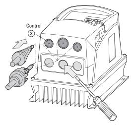
Figure 47. Punching out the knockouts (Example)
