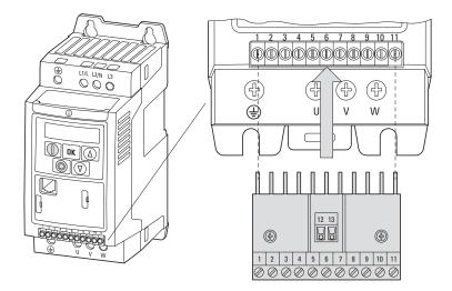
Figure 79. Connecting DXC... to the control signal terminals on the VSC
