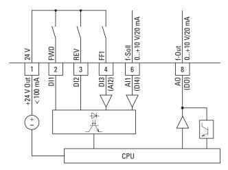
Figure 54. Control signal terminals (D = digital / A = analog)
