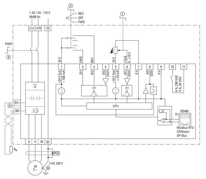
Figure 65. Block diagram VSC1D...NxA6S...
