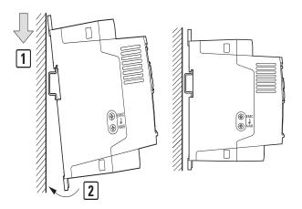
Figure 29. Fixing on a mounting rail
