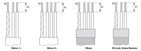
Figure 43. Stripping lengths in the power section
