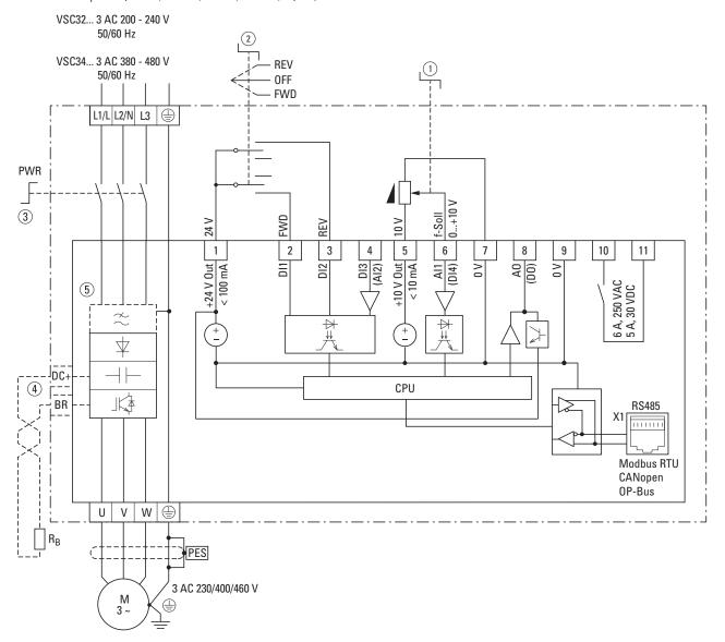
Figure 69. Block diagram VSC32...A6S..., VSC34...A6S...
