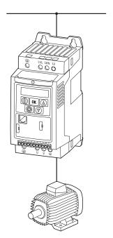
Figure 41. Connection in power section (schematic)
