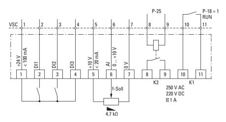
Figure 83. Block diagram DXC-EXT-2RO
