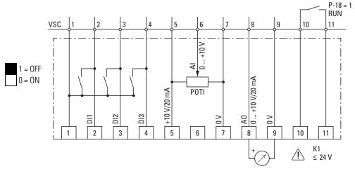
Figure 87. Block diagram DXC-EXT-LOCSIM simulator
