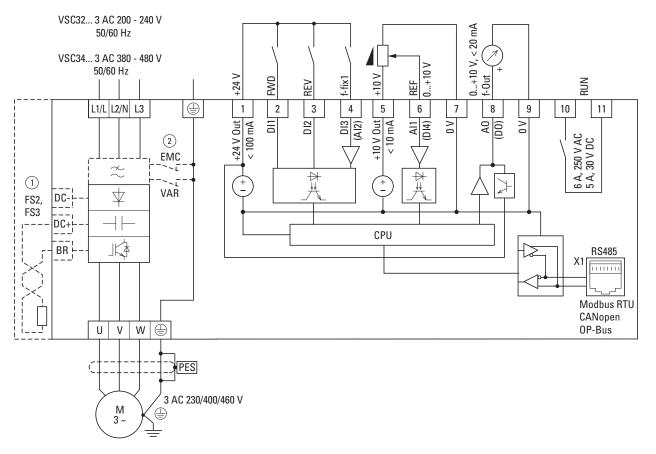
Figure 63. Block diagram VSC32... and VSC34... in frame sizes FS1, FS2 and FS3
