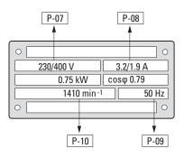
Figure 75. Motor rating plate, P-08 = 1.9 A at 400 V
