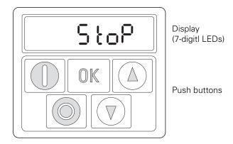
Figure 72. Operating unit view (example VSC...A20...)
