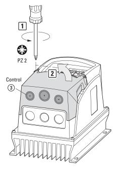
Figure 42. Removing the lower housing cover
