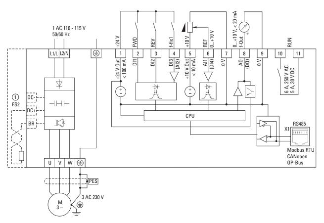
Figure 61. Block diagram VSC1D...Nx-...
