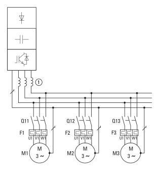
Figure 19. Example: Parallel connection of several motors to one variable speed drive
