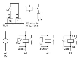
Figure 57. Connection examples with suppressor circuit
