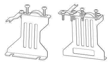
Figure 38. DX-EMC-MNT-...N (left), net and DX-EMC-MNT-...M (right), motor, cable brackets
