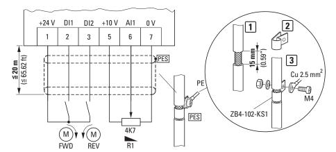
Figure 52. Simple connection example
