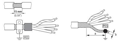
Figure 45. Screened connection cable in motor circuit
