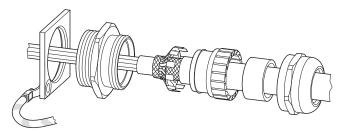
Figure 50. Example: diagram of EMC gland assembly
