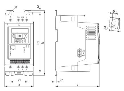
Figure 76. Dimensions for VSC with IP20 degree of protection (NEMA 0)
