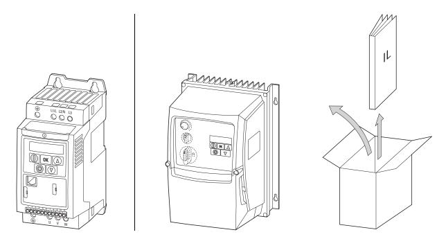
Figure 3. Equipment supplied (example: devices with IP20 / IP66 degree of protection with instruction leaflet)
