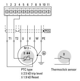
Figure 60. Thermistor connection
