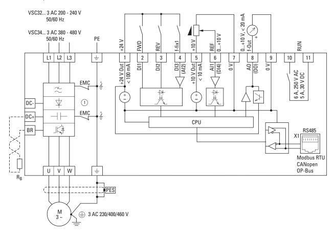
Figure 64. Block diagram VSC32... and VSC34... in frame size FS4
