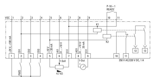
Figure 85. Block diagram DXC-EXT-2RO1AO
