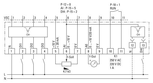
Figure 81. Block diagram DXC-EXT-IO110 and DXC-EXT-IO230
