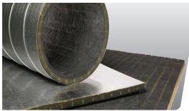
Spiracoustic Plus® is a fiberglass insulation designed to line spiral ducts. It has factory-made, evenly spaced kerfs to allow the material to easily conform to the inside diameter of spiral air ducts. The airstream surface and transverse edges are protected with JM's factory-applied Permacote coating. Spiracoustic Plus can save time and reduce weight when compared to some double-wall systems.
