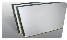
Diffuser Board is a 4pcf density fiberglass board insulation designed to insulate air diffusers and register boxes. The glass mat airstream surface provides a smooth interior that offers minimal resistance to airflow.
