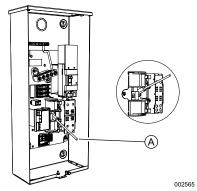
Figure 3-11. Typical Manual Transfer Switch Operation
