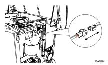
Figure 4-9. Disconnecting Battery Charger Cable
