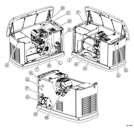
Figure 2-3. 20 kW-26 kW-Components and Control Locations
