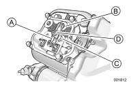
Figure 4-7. Valve Clearance Adjustment (10 kW)
