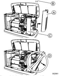
Figure 3-3. Intake Side Panel Removal
