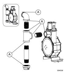
Figure 4-12. Connection Points to Leak Check
