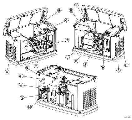
Figure 2-1. 10 kW—Components and Control Locations
