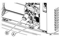
Figure 4-3. Oil Filter and Drain Location (20-26 kW)
