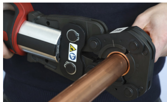
3. Complete the joint with the press tool
