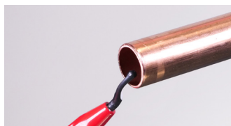
3. Use a pencil type deburrer on internal edges
