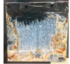
Builder's Best black metal roof caps begin with galvanized steel which has some corrosion protection. Our high performance polyester powder coating showed very little corrosion. The leading brand uses cold rolled steel, which has no corrosion protection. Their paint coat showed some corrosion. Competitor X uses galvanized steel, which has some corrosion protection, however, the paint they used failed.
